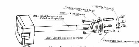
● Metal flange installation diagram
