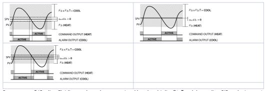
Parameter co.F (Cooling Fluid) pre-selects the proportional band multiplier  $P.b.\Pi$  and the cooling PID cycle time c.c.E according to cooling fluid type:
